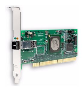
Designed and deployed by major server and storage OEMs, QLogic's SANblade QLA2340 and QLA2340L host bus adapters (HBAs) offer the ultimate in performance: 2-Gb Fibre Channel combined with 64-bit, 133-MHz PCI-X. Eliminating traditional host bottlenecks that impede the high performance of 2-Gb Fibre Channel, this union of the fastest I/O and host technologies creates the perfect balanced solution.
