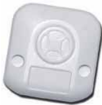
The TiMax Tracker radar tag, 1" square
