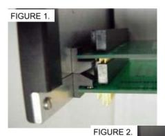
2. Then squeeze the HW-PC104-EXT's handle, which will pull the blocks apart and thus separate the boards (Figures 2 & 3).
