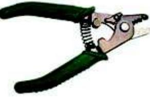
A green-handled fiber stripper with a metal head and a spring mechanism.              |
