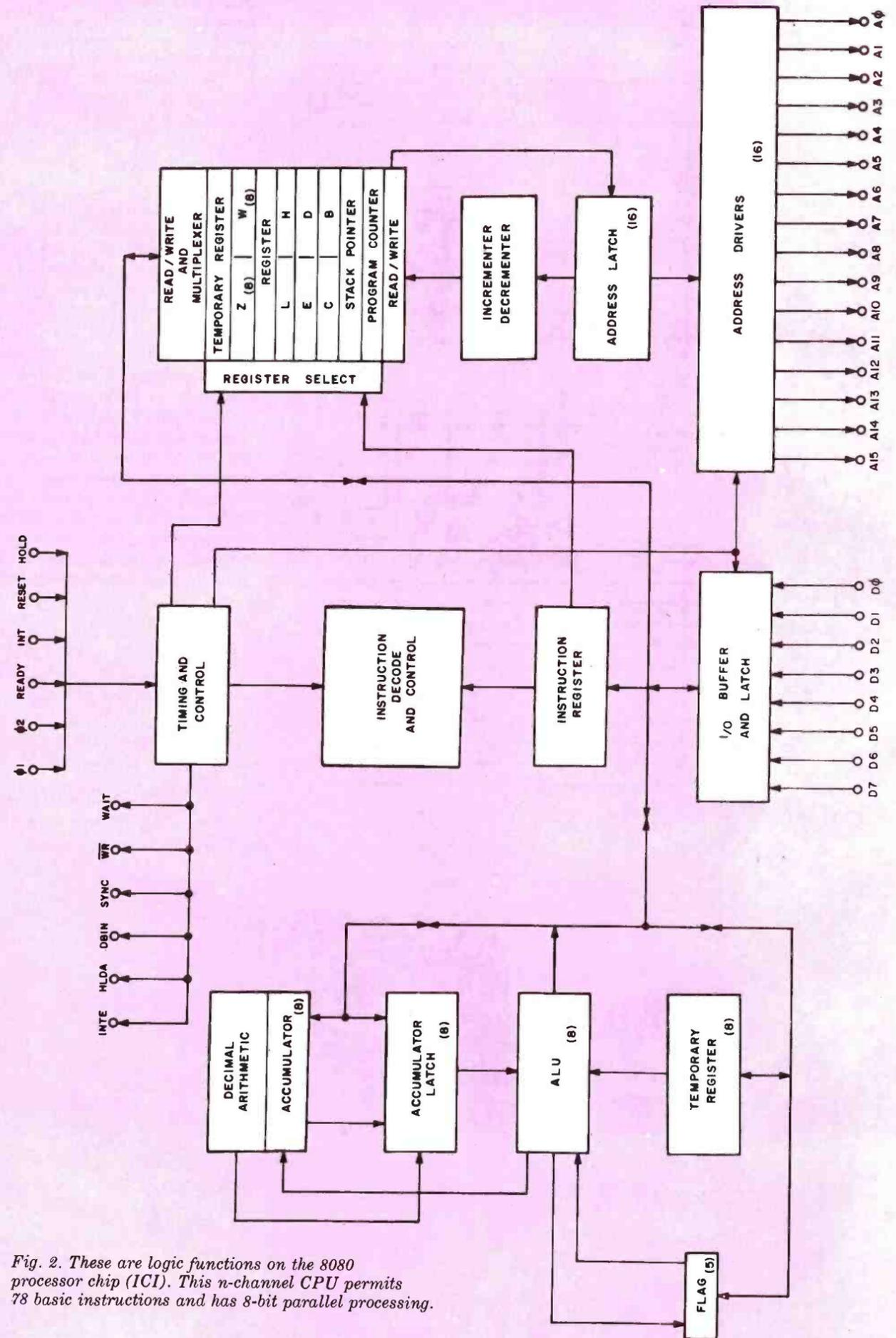
Fig. 2. These are logic functions on the 8080 processor chip (IC1). This n-channel CPU permits 78 basic instructions and has 8-bit parallel processing.
