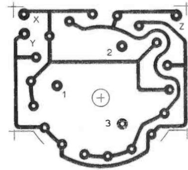
Fig. 2. Foil pattern for main pc board is at left, with component layout at right. Foil pattern above is for rotary switch.
