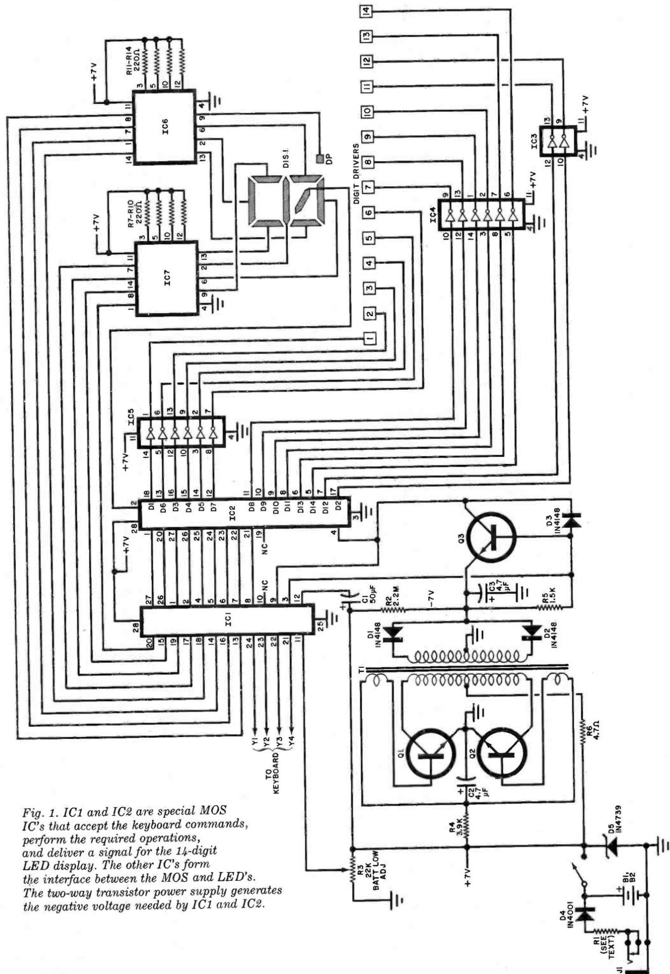
Fig. 1. IC1 and IC2 are special MOS IC's that accept the keyboard commands, perform the required operations, and deliver a signal for the 14-digit LED display. The other IC's form the interface between the MOS and LED's. The two-way transistor power supply generates the negative voltage needed by IC1 and IC2.
