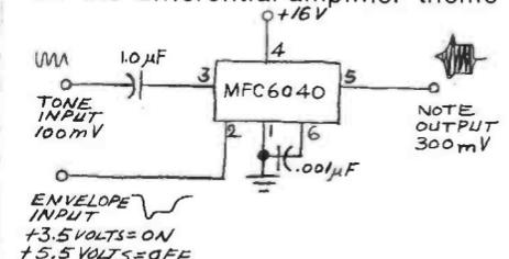
Fig. 5. Gain block envelope shaper.
