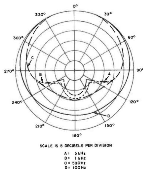
Fig. 2. Cardioid pickup patterns at four different frequencies.
