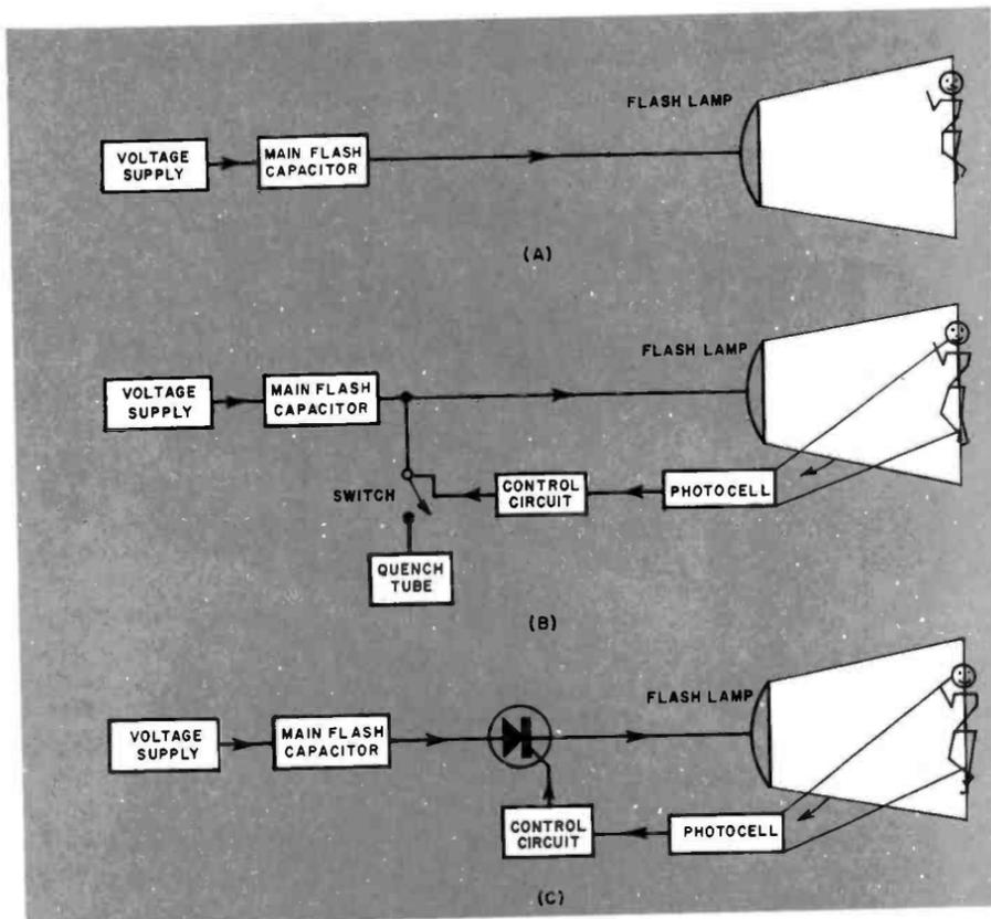
Three greatly simplified block diagrams show the major components of the various types of electronic flashers. At (A), a manual unit is the least complex. Diagram (B) shows how a photocell is added with control circuit and quench tube to dump surplus energy. At (C), a thyristor unit adds an SCR to trap voltage from the main flash capacitor.
