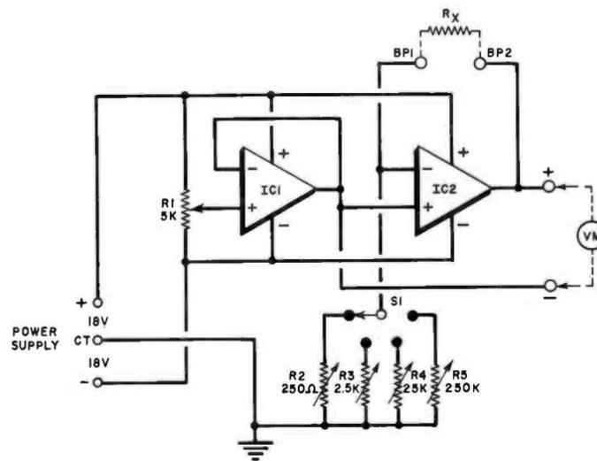
Linear scale ohmmeter uses two integrated circuits. When the circuit is properly balanced (via range switch and potentiometers), the meter reading is proportional to the unknown resistor.
