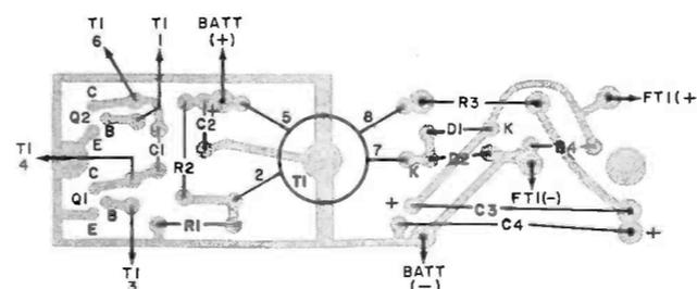
Fig. 2. Foil pattern is above, component placement, left.
