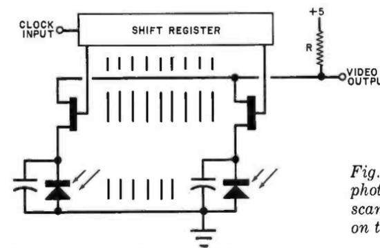
Fig. 10. Self-scanned photodiode array is scanned by transistors on the IC chip.
