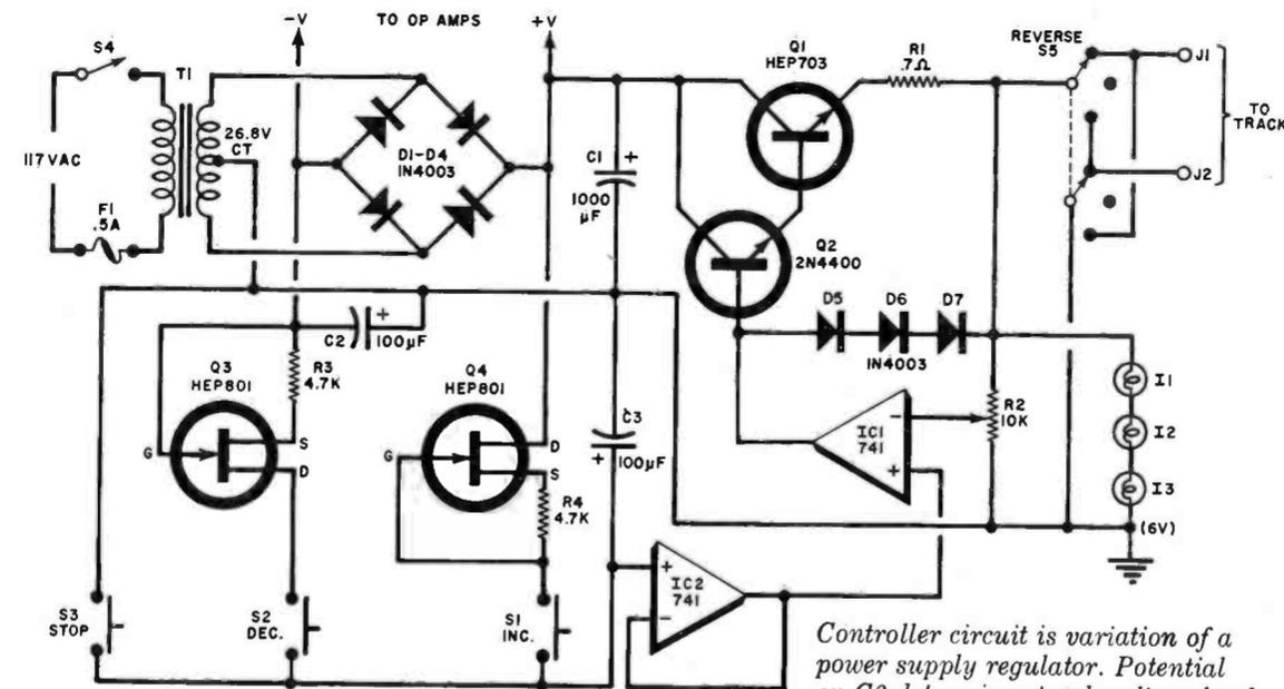
Controller circuit is variation of a power supply regulator. Potential on *C3* determines track voltage level.
