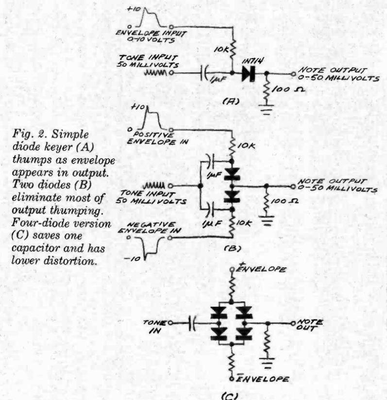
*Fig. 2. Simple diode keyer (A) thumps as envelope appears in output. Two diodes (B) eliminate most of output thumping. Four-diode version (C) saves one capacitor and has lower distortion.*
