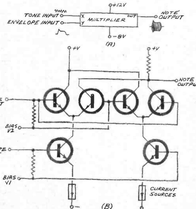
Fig. 4 (A) are typical connections for 4-quadrant multiplier. Key internal circuitry is shown at (B).
