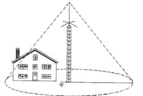
Fig. 3. A metal antenna tower, properly grounded, provides a cone of protection for the house.
