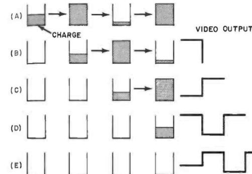
Fig. 8. Charges in CCD array are transferred from left to right to produce a video output.
