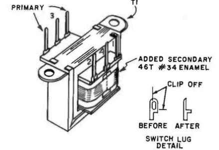
Fig. 3. Add a winding and terminals to the transformer and alter switch lugs as shown.
