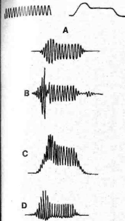
**What a Keyer Does.** Any keying circuit must simply control the gain of the tones fed through it. In Fig. 1 are shown some good and some bad things keyers do. The keyer must behave as a linear, electrically bilateral variable resistor. Ideally, it must introduce no coloration or significant distortion of its own (Fig. 1A).
