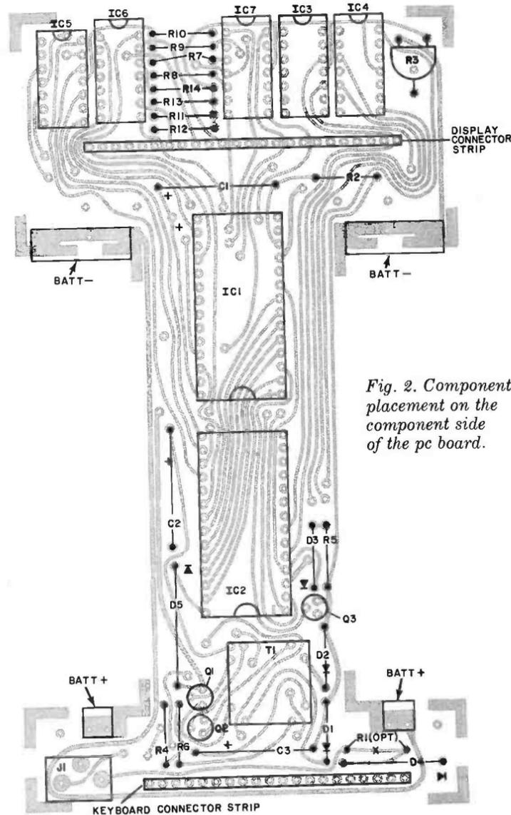
Fig. 2. Component placement on the component side of the pc board.
