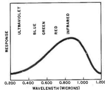
Fig. 7. Spectral response of silicon to various colors of light.
