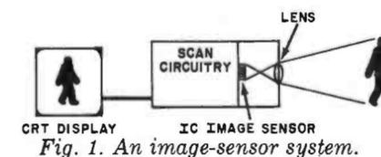
A linear array can be used to produce a two-dimensional picture, but only one line at a time as the image
