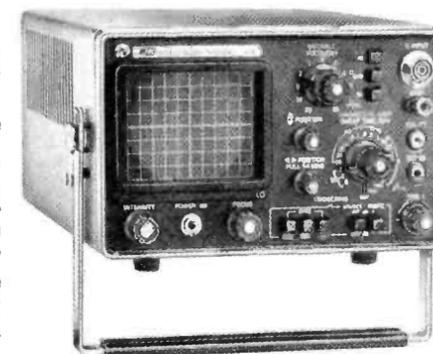
available. Rise time of the vertical amplifier is 35 nanoseconds, overshoot is 3% or less, and the input impedance is 1 megohm shunted by 35 pF. The 1431 is supplied with a handle/tilt stand, Mylar vector overlay (so the unit can be used as a vectorscope), but less probe. It is \$399.00.
