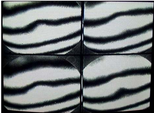
Figure 5 Real-time video display of four simultaneous interferograms
