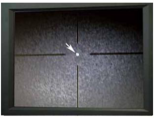
Figure 2. Both the test and reference beams should pass through the crosshairs on the Alignment Monitor.
