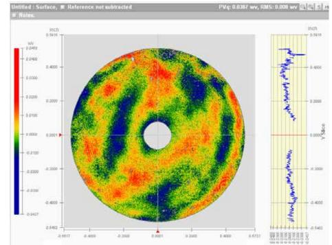
Figure 3. Homogeneity of a glass disk measured using the FizCam 2000.
