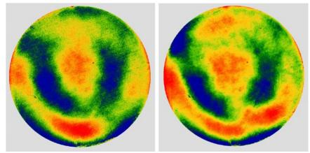
Figure 3. Using Gain 8 results in significant measurement noise (left). Lowering the Gain and increasing the Exposure (right) reduces noise.
