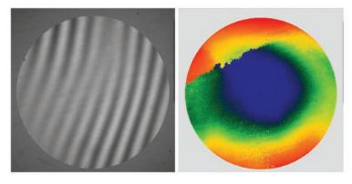
Figure 2. A long Exposure time washes out the fringes (left), leading to unwrapping errors (right). Raise the Gain and lower the Exposure to eliminate this condition.
