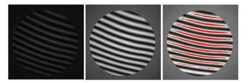
Figure 1. Interference fringes with, a) low intensity, b) good intensity, c) intensity exceeding the camera limit (saturated pixels in red).
