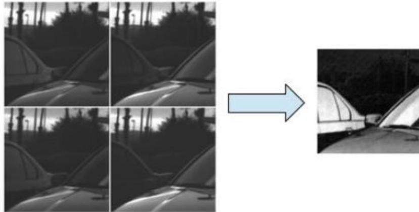
Figure 7. Parsed pixelated camera polarization images shown on the left with two cars in the foreground and trees and shrubs in the background. On the right the corresponding DoLP image clearly discriminates the cars from the background scenery.
