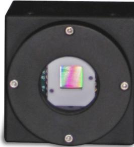
Figure 2. Compact 1Mpixel micropolarizer camera (57x57x46mm) with C-mount.
