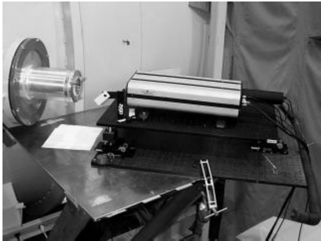
Figure 1 PhaseCam in Operation at the Thermal Vacuum Chamber
