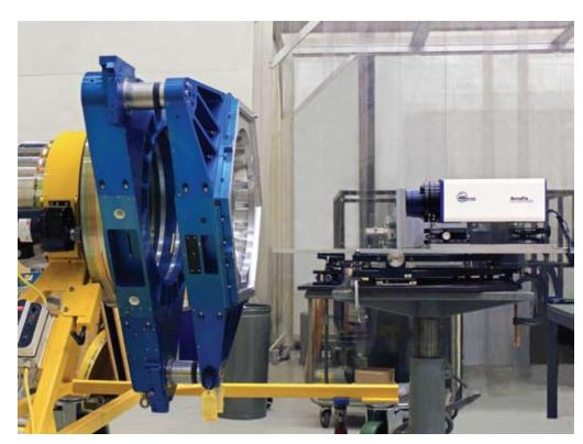
Figure 3. Vibration-Insensitive AccFiz Interferometer at NOAO's Optics Shop facility, shown here measuring components for the WIYN telescope's One Degree Imager.
