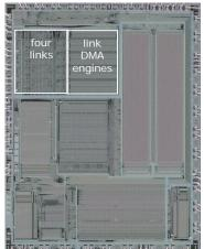
Figure 3: Chip photo of the T800 transputer, showing the area taken by the serial links
