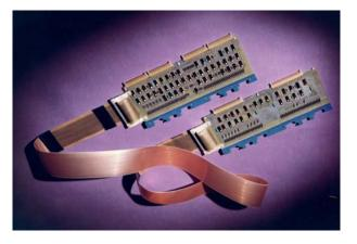
Figure 1. Standard Interface on Modular One Computer
