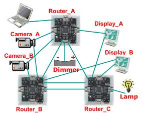
Figure 11. A dimmer switch and lamp are added as examples of simple devices that do not require a large overhead to be used in the SpaceWire Plug and Play network.
