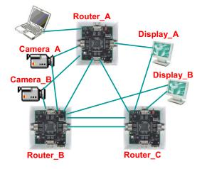
Figure 10.Additional SpaceWire links are added to provide further redundancy and fault-tolerance, allowing removal of power from Router B or Router C
