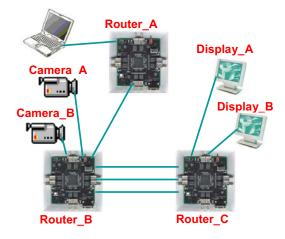
Figure 7. When a redundant link is added, traffic is shared between the redundant set of links.
