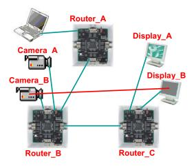
Figure 5. Adding another camera and display — not enough bandwidth
