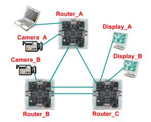
Figure 9. Devices can be moved around the network. In this case Camera A is moved from Router B to Router A, and the camera's images are displayed just as before
