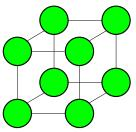
19<sup>th</sup> century, which achieves ten nodes with three ports per node and with a maximum path-length of two between any nodes. Compare this with a cube, which has eight nodes, again has three ports per node, but has a path length of three between nodes on opposite corners — fewer nodes than Petersen yet a longer path length — but possibly easier to build physically.
