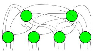
The cost of needing six eight-port switches to make a single full-bandwidth 16-port switch makes a strong argument for building switches with as many ports as possible. But, as we shall consider next, a single large switch is a large single point of failure.
