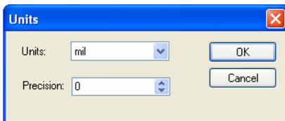
For each type of units, you can specify a **Precision:**. This is the number of decimal places displayed; the value is simply rounded to the nearest last digit.
