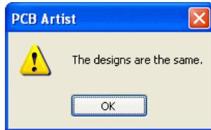
If differences are found, Notepad will be run to view a detailed report. The report will give you a list of changes that would have to be made to the PCB in order to make it match the schematic (the schematic always being the 'master'). You can then perform these changes automatically by selecting the **Yes** button on the dialog.
