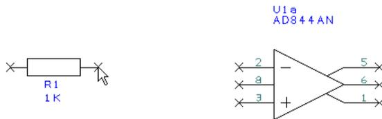
Click and drag (keeping the mouse button pressed down) off pin 2 of R1, this will start a new connection. Move the mouse over U1a pin 2 and single click to finish.
