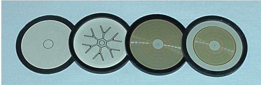
**Figure 1.** Si-Wafers  $\varnothing$ 51 mm for  $di/dt < 0.1kA/ms$ ,  $1kA/ms$ ,  $18kA/ms$  and  $15kA/ms$ .
