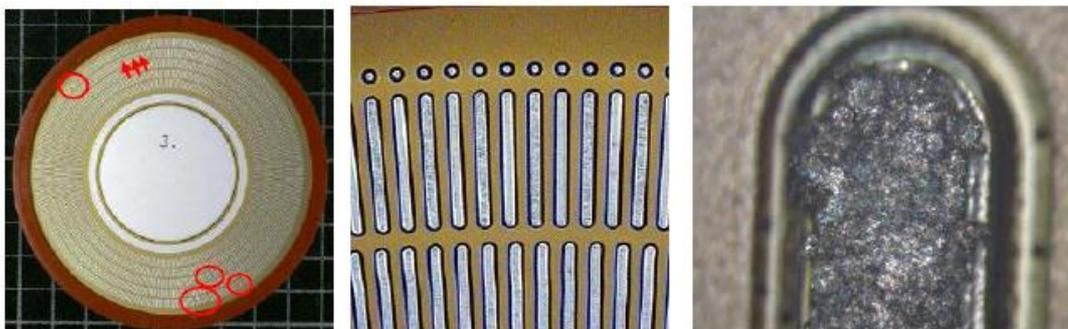
**Figure 10:** Cathode side of wafer, middle picture shows contact finger arrangement, right picture shows burned contact finger with almost an cathode-anode short
