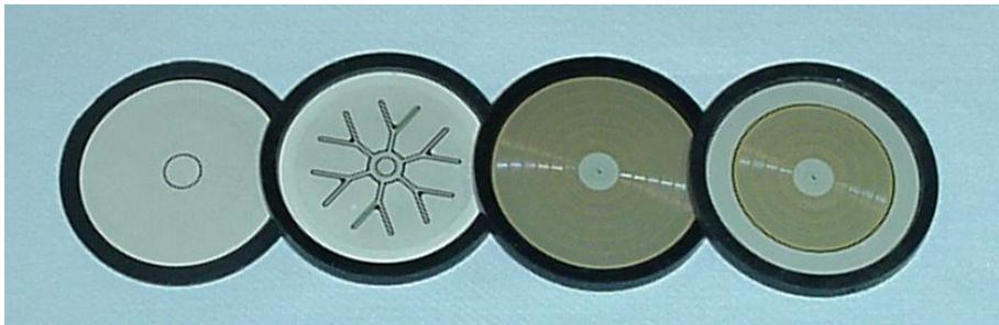
**Figure 1.** Si-Wafers Ø51 mm for  $di/dt < 0.1kA/\mu s$ ,  $1kA/\mu s$ ,  $18kA/\mu s$  and  $15kA/\mu s$ .
