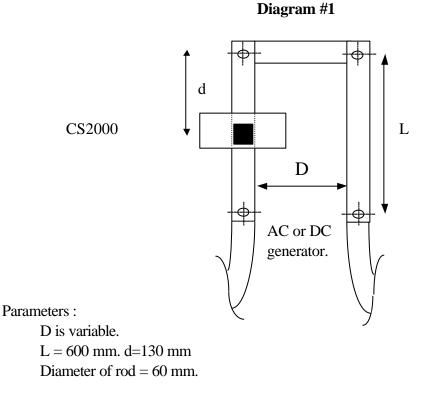
We used this configuration to realise the accuracy map, given in page 7 and 8. We made turn the sensor of each  $15^{\circ}$  angle, and we move the distance D in order to got an accuracy of 0.5%. We realize it for AC and DC current. The minimum distance (D) is 140 mm.
