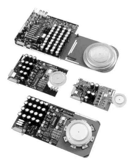
Figure 1: Photograph of reverse conducting IGCTs
