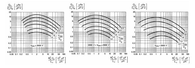
Fig 7 Curves for determining the optimum RC snubber values of ABB phase control thyristors. The curves are valid for thyristors with  $V_{RRM}$  ratings below 2000 V (a), between 2000 and 3000 V (b) and above 3000 V (c). For diodes, similar curves apply but they depend somewhat more on the specifics of the design of the individual part number.
