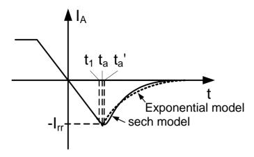
Fig 4 Comparison of exponential and sech models, adjusted to exhibit the same di/dt, Q<sub>rr</sub> and I<sub>rr</sub>
