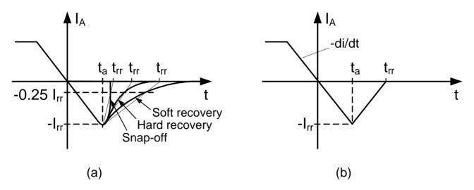
Fig 3 Types of reverse recovery waveforms (a) and simplification by a triangular model (b)
