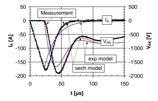
Fig 6 Turn-off transients for a 5STP 18L4200 thyristor at 125 °C and -7.9 A/ $\mu$ s with a snubber of 10  $\Omega$ /1.0  $\mu$ F and a reverse voltage of about -800 V. The measured waveform is compared with model transients adjusted for equal di/dt,  $Q_{rr}$  and  $I_{rr}$ .
