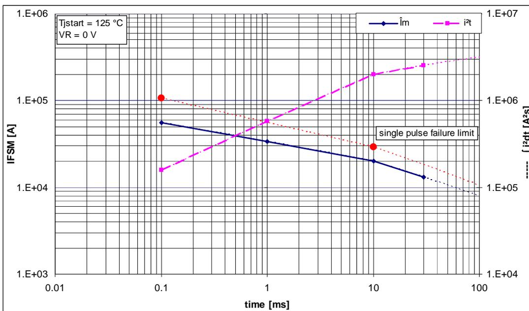
Figure 6 Surge on-state current vs. pulse length, half-sine wave for 5SNA 2400E170100
