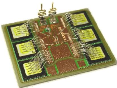
Figure 3 Layout of a substrate to optimise current sharing between the diode dies.
