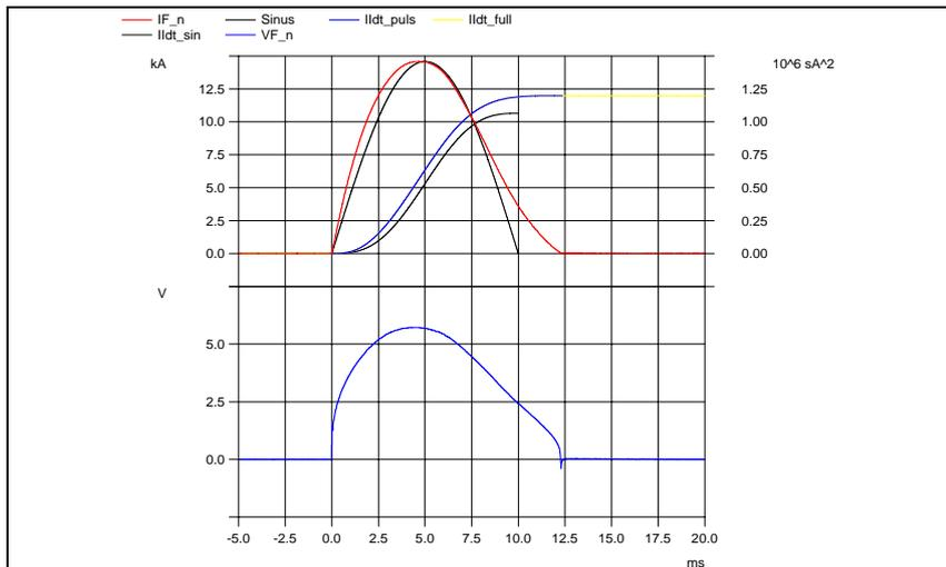
Figure 5 Typical wave forms at surge current testing
