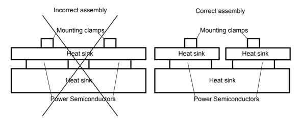
Figure 4. Devices should be individually clamped.
