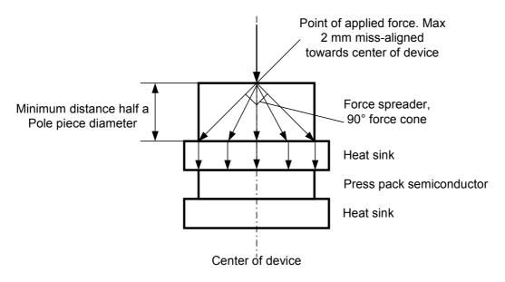
Figure 2. Recommended application of the mounting force.
