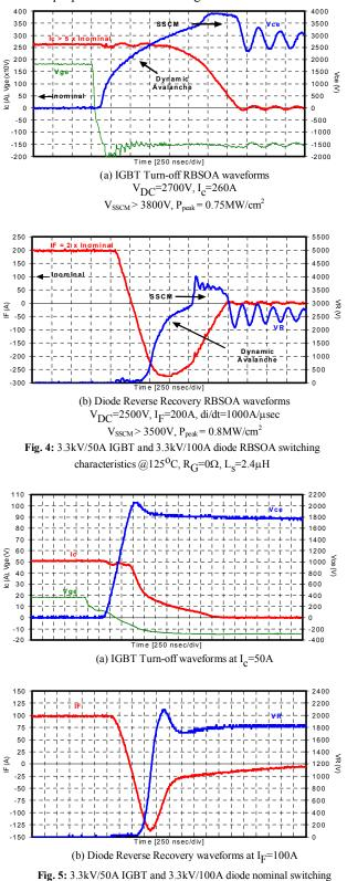
characteristics @125°C,  $V_{DC}$  =1800V,  $R_G$ =33 $\Omega$ ,  $L_s$ =2.4 $\mu$ H Typical nominal condition losses are outlined in table (1) along with the new 4.5kV and 6.5kV IGBTs. All devices exhibit a positive temperature coefficient at rated currents. To demonstrate a similar RBSOA performance for higher
