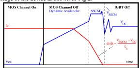
Fig. 2: IGBT SOA turn-off waveforms including SSCM
