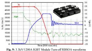
V<sub>DC</sub>=2600V, I<sub>c</sub>=5000A, 125<sup>o</sup>C, R<sub>G</sub>=1.5Ω, L<sub>s</sub>=280nH
