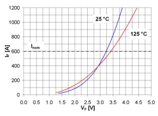
(b) Forward characteristics of the 6.5kV SPT-diode
