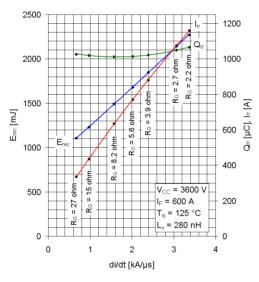
Figure 9. 6.5kV/600A HV-HiPak<sup>TM</sup> E<sub>rec</sub>, I<sub>rr</sub>, Q<sub>rr</sub> vs. di/dt curves.
