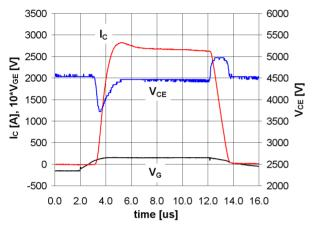
Figure 13. 6500V/600A HV-HiPak<sup>TM</sup> SCSOA characteristics.  $V_{CC}=4500V, R_{Goff}=3.9\Omega, V_{GE}=15V, L_{\sigma}=300nH, T_{j}=125$  °C
