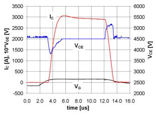
Figure 12. 6500V/600A HV-HiPak<sup>TM</sup> SCSOA characteristics.  $V_{CC} = 4500V$ ,  $R_{Goff} = 3.9\Omega$ ,  $V_{GE} = 15V$ ,  $L_{\sigma} = 300nH$ ,  $T_j = 25$  °C
