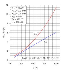
Figure 6. 6.5kV/600A HV-HiPak<sup>TM</sup>  $E_{on}$  and  $E_{off}$  vs.  $I_c$  losses curves.
