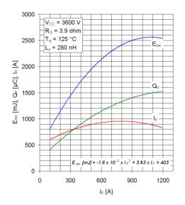
Figure 7. 6.5kV/600A HV-HiPak<sup>TM</sup> Erec, Irr, Qrr vs. IF losses curves.
