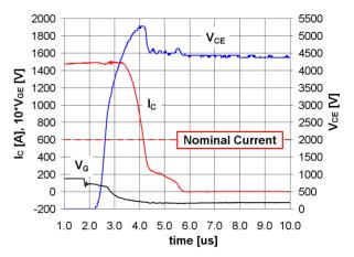
Figure 10. 6500V/600A HV-HiPak<sup>TM</sup> IGBT turn-off characteristics under high SOA conditions. V<sub>CC</sub> = 4400V, I<sub>C</sub> = 1500A, R<sub>Goff</sub> = 1.5 $\Omega$ , L<sub> $\sigma$ </sub> = 300nH, T<sub>i</sub> = 125 °C.
