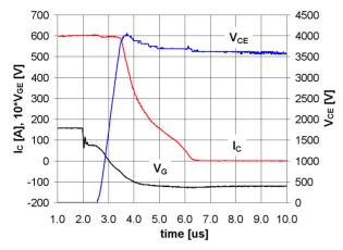
Figure 3. 6500V/600A HV-HiPak<sup>TM</sup> IGBT nominal turn-off waveforms.  $V_{CC} = 3600V, I_C = 600A, R_{Goff} = 2.7\Omega, L_{\sigma} = 300nH, T_j = 125 \text{ °C}.$
