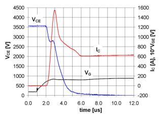
Figure 4. 6500V/600A HV-HiPak<sup>TM</sup> IGBT turn-on waveforms at nominal condition. V<sub>CC</sub> = 3600V, I<sub>C</sub> = 600A, R<sub>Gon</sub> = 3.9 $\Omega$ , L<sub> $\sigma$ </sub> = 300nH, T<sub>j</sub> = 125 °C.
