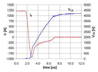
$\begin{array}{l} \mbox{Figure 11. 6500V/600A HV-HiPak^{TM} diode reverse recovery} \\ \mbox{characteristics under SOA stress. } V_{CC} = 4400V, I_F = 1200A, R_{Gon} = 3.9\Omega, \\ \mbox{} L_{\sigma} = 300nH, T_j = 125 \ ^{\circ}C \end{array}$
