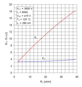
Figure 8. 6.5kV/600A HV-HiPak<sup>TM</sup>  $E_{on}$  and  $E_{off}$  vs.  $R_g$  curves.
