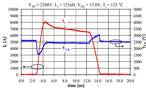
Figure 10: EP-IGBT short-circuit test at 125 °C.
