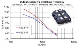
Figure 10: Inverter output current vs. Frequency for 3300V/1200A modules.
