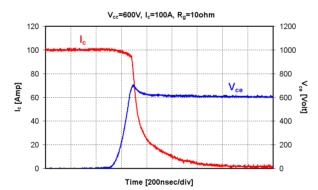
Figure 5: 1200V/100A SPT<sup>+</sup> IGBT turn-off waveforms at 125°C.
