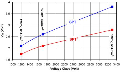
Figure 1: SPT vs. SPT<sup>+</sup> IGBT on-state losses at the indicated current densities for the 1200V, 1700V and 3300V chips at 125°C.
