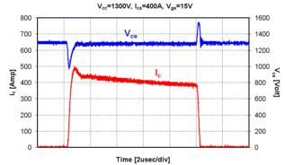
Figure 8: 1700V/100A SPT<sup>+</sup> IGBT SCSOA waveforms at 25°C.
