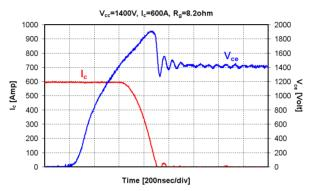
Figure 7: 1700V/100A SPT<sup>+</sup> IGBT RBSOA waveforms at 125°C.
