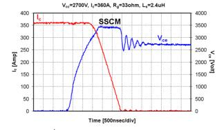
Figure 9: 3.3kV/50A SPT<sup>+</sup> IGBT chip RBSOA waveforms at 125°C with "SSCM".
