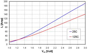
Figure 4: 1700V/100A SPT<sup>+</sup> IGBT on-state characteristics at 25°C and 125°C.
