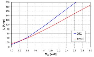
Figure 3: 1200V/100A SPT<sup>+</sup> IGBT on-state characteristics at 25°C and 125°C.
