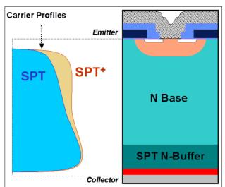
Figure 2: SPT<sup>+</sup> planar IGBT enhanced carrier profile compared to the SPT standard profile.
