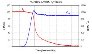
Figure 6: 1700V/100A SPT<sup>+</sup> IGBT turn-off waveforms at 125°C.
