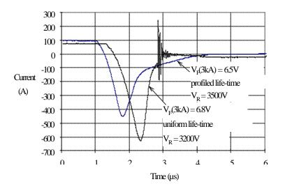
Figure 11: Comparison of different lifetime technologies in 4.5 kV snubber diodes. Note the different source voltages.
