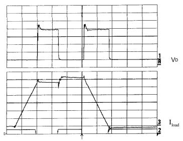
Figure 5: Current and voltage waveforms of a buffer layer GTO (ABB type 5SGF 30J4502) during frequency testing. In the upper part the voltage of the DUT is shown. In the lower part the current in the load is shown. (t: 200µs/div, I: 500A/div, U: 1kV/div)
