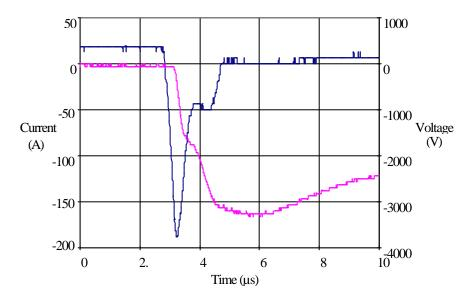
Figure 12: 5SDF 03D4501in Undeland/Marquardt circuit,  $I_F = 10$  A,  $V_{dc} = 3500$  V, T = 110 °C
