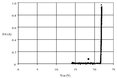
Figure 6: Reverse gate characteristic of RC-GTO
