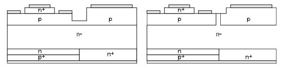
Figure 3: Comparison of resistive separation with pnp separation of a GTO and integrated freewheeling diode. The advantages of the pnp separation are very low gate leakage currents,  $I_{GRM}$ , and high blocking stability.
