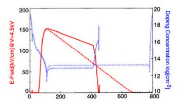
Figure 1: Comparison of doping profiles (grey) and electric field (black) of a non punch-through (- -) and a buffer layer GTO (—). The electric field is calculated at a blocking voltage of 4.5 kV. It can be seen that the thickness of the wafer can be reduced by roughly a factor of two.
