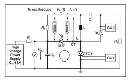
Figure 10: Test circuit to evaluate the behaviour of snubber diodes under worst case conditions The commutation loop is drawn in **bold**
