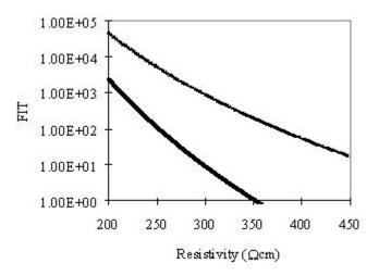
Figure 2: Calculated failures in time due to cosmic radiation at sea level for a buffer layer GTO with an n-base thickness of 400  $\mu$ m [3]. The calculation assumes dc link voltages of 2.2 kV (—) and 2.8 kV(- -) respectively. The silicon area is 60 cm<sup>2</sup>.
