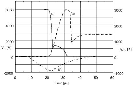
Figure 7: Turn-off waveforms of a 6 kV buffer layer GTO. The on-state of this device is 3.25 V at 3 kA and 110 °C. The turn-off conditions are Cs =  $2.66 \,\mu$ F, Ls  $\approx 250 \,\text{nH} \,\text{di}_g/\text{dt} = 70 \,\text{A}/\mu$ s, T =  $110 \,$  °C.
