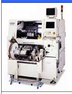
Our SMT lines use advanced Vision recognition to insure repeatability and placement accuracy. They can place components to  $\pm$ 0.075mm (0.0029 in.) with a repeatability of  $\pm$ 0.025mm (0.001 in.)
