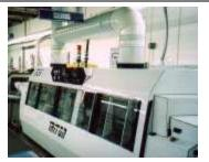
In-line de-ionized aqueous cleaning system insures that your product is thoroughly clean and dry. After cleaning our Ionic Contamination tester incorporates the most advanced innovations for high speed non-destructive testing.
