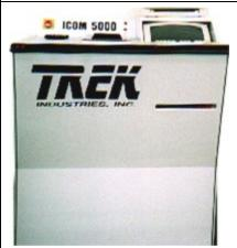
Our Ionic Contamination Tester insures that any residual contamination is at levels that are within our customers' specifications.
