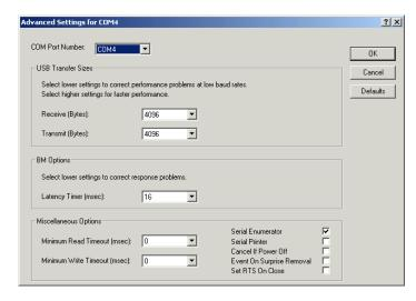
The Advanced Settings window allows the COM port number assigned to the probe to be changed.
