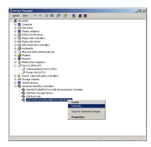
Next click the [+] box to expand the Universal Serial Bus controllers branch then select the USB Serial Converter/ABACUS Optical Probe entry. Right-click to get the context menu and then select 'Uninstall'.
