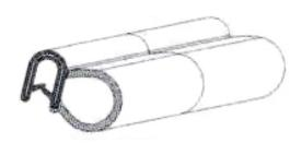
Sealing profiles as a combination between PVC edge trim and sponge rubber can have up to two glued joints.
