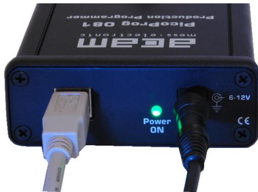
**Please note:** when plugging in the PicoProg Ø81 you need to make sure that it is power supplied by the external wall power supply unit (green LED on). The device is not supplied by USB!
