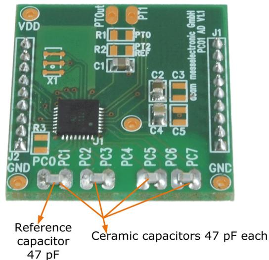
In the process of evaluation, when you are comfortable with interpreting the measurement results from the chip, these fixed capacitors can be replaced with the actual capacitive sensors of your application.
