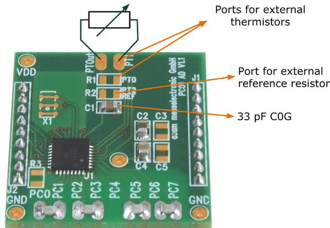
However, there is a possibility to connect the reference resistor and the thermistor externally to the chip too. In case of external resistors, the temperature-stable reference resistor ought to be connected at port PT2REF on the plug-in module. The module allows you to connect the external thermistor used for temperature measurement at port PT0 or PT1.
