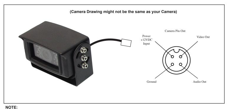
This camera is designed with water resistance technology only. These camera are not designed to be submerged in water.
