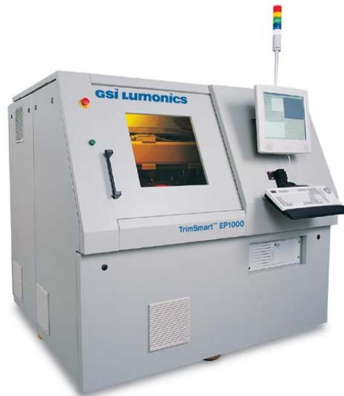
Fig.1: GSI Lumonics EP laser trimmer
