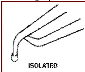
The isolated edge sensor is an SPST NC switch, which is electrically isolated from the device surface by a jewel bead.
