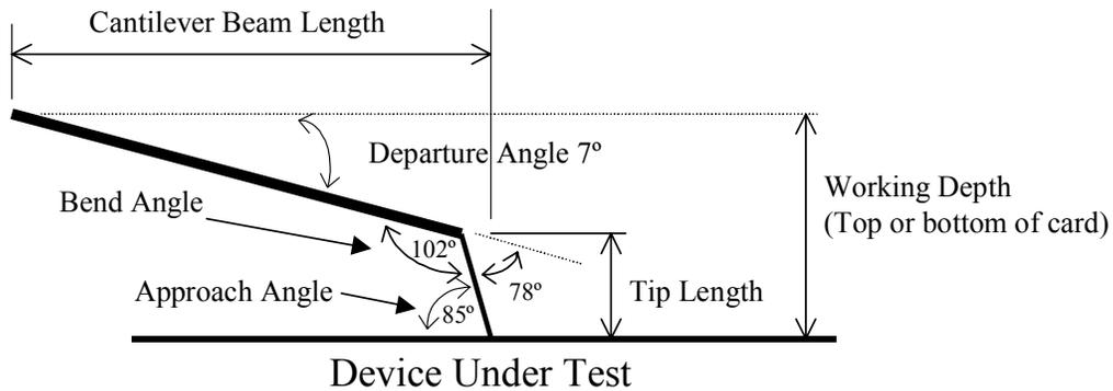
Where very fine geometries need to be probed another possibility would be to use a special tip bend of 83°, which would result in a 90°-approach angle (less scrub) to the bond pad, assuming standard overdrive.
