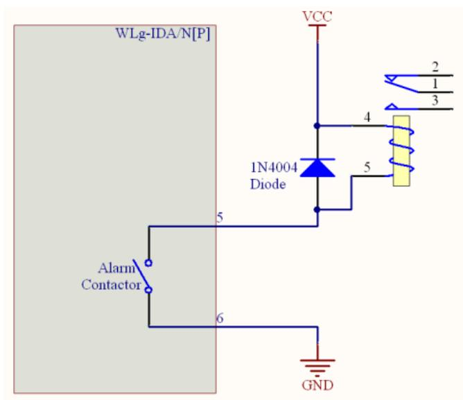
The alarm contact can switch a 60V maximum voltage for a 150 mA maximum current.
