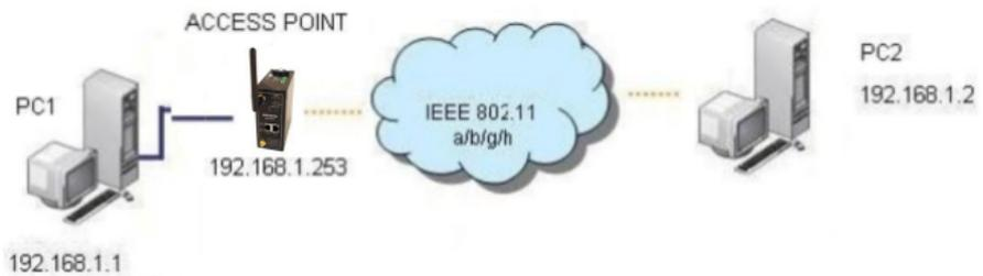
Setup PC2 Wireless network interface according to the default parameters of the ACKSYS AP device (802.11b/g, SSID ACKSYS, no security).
