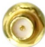
**If your product includes the H4(400mW) option, it is mandatory to use a second antenna on the auxiliary antenna connector or a 50 Ohms RP-SMA type antenna terminator.**
