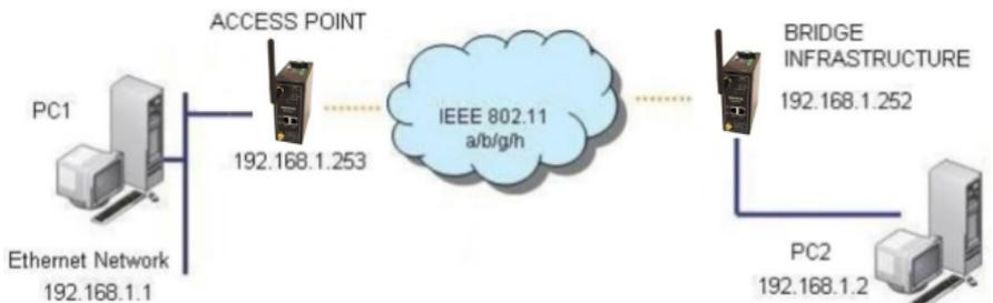
Setup the ACKSYS device connected to PC2 in Bridge mode.
