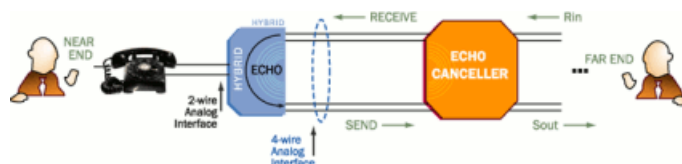
Figure 1. The hybrid circuit in the telephone network that causes the voice signal to be reflected. Also shown is an echo canceller that is used to cancel the reflection.
