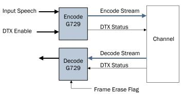
The decoder is also fed a frame erase flag, which is an indication that the decode stream has temporarily been corrupted. The decoder is able to "smooth over" the output, doing its best to conceal the loss of data and minimize the loss in voice quality. This process is known as packet loss concealment (PLC). It works surprisingly well even under high packet loss rates.
