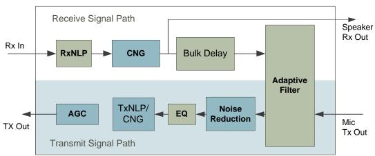
The terms Rx (Receive) and Tx (Transmit) may be confusing at first because both the receive and transmit paths have inputs and outputs. The names receive and transmit are used from the point-of-view of the person at the speaker/microphone side.
