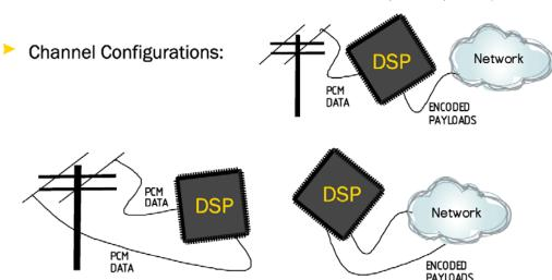
Each G.PAK DSP supports a fixed number of channels. The number of channels available in a DSP is dependent on the DSP type and the capabilities selected at build time.
