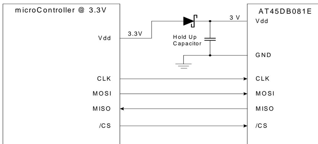
**Figure 1. Test Circuit**
