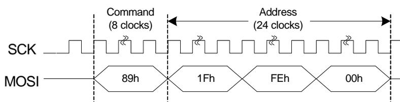
Figure 6. SRAM Buffer 2 to Flash Memory Transfer
