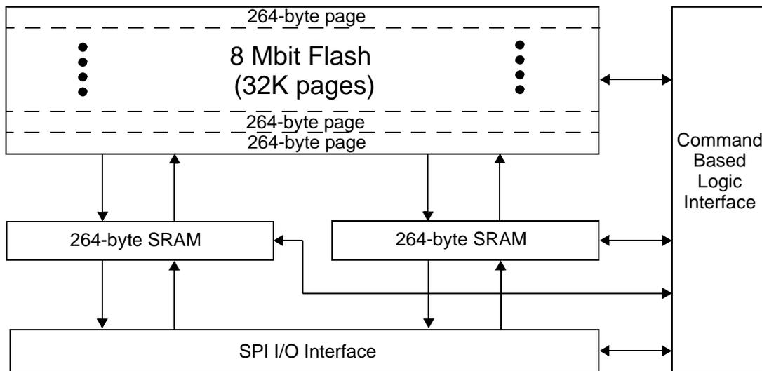
Figure 2. E-Series DataFlash Simplified Block Diagram
