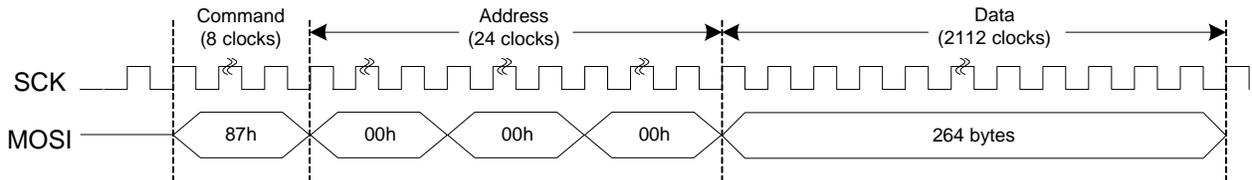
**Figure 5. Transferring Data to the Buffer 2 SRAM**
