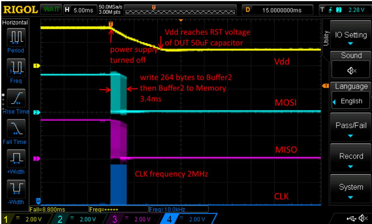
Figure 4. Oscilloscope Output of Experiment 2
