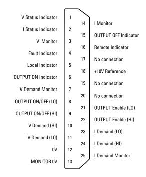
All logical Indicators are open collector outputs rated at 16V (max) in the off state. An internal  $100\Omega$  resistor is connected in series with the open collector transistor. The pull down voltage is 0.9V plus the internal resistor drop. The rated current is 10mA.
