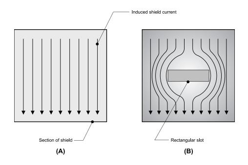
figure 6 current distribution with and without a hole
