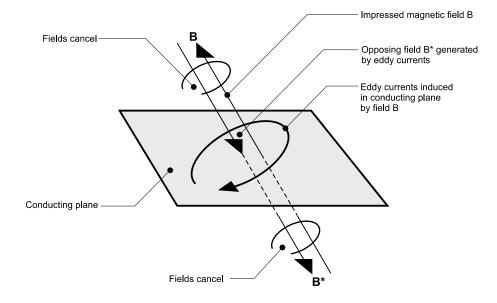
figure 5 time-varying magnetic field inducing currents
