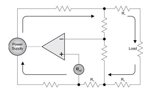
figure 2 regulated power supply (actual circuit)
