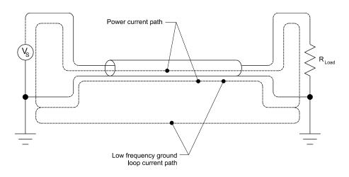
figure 8 power source connected to a remote load with a coaxial cable
