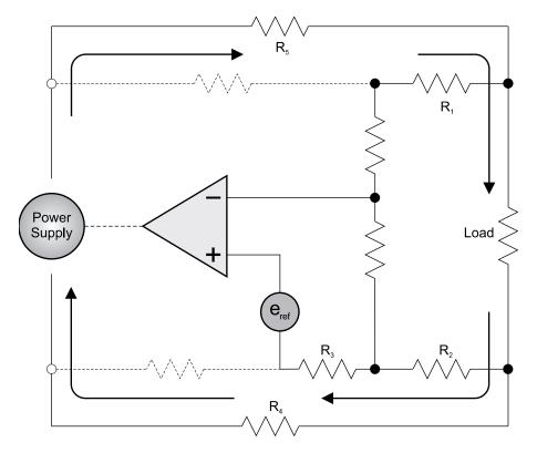
figure 3 regulated power supply with separate load current path
