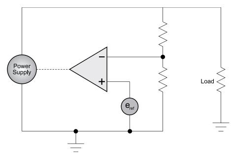
figure 1 regulated power supply (supposed circuit)
