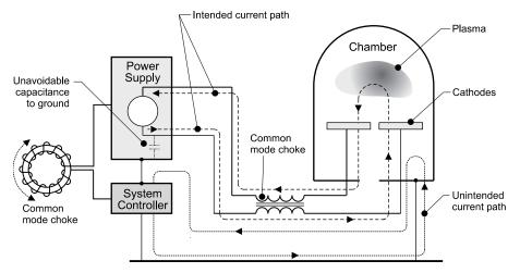
figure 13 common-mode choke
