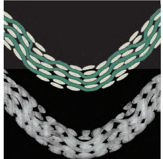
fiber locations from forming simulation
