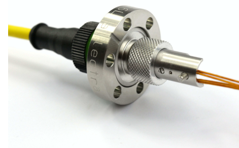
M12 feedthrough, seen from the vacuum side, with connectors. The UHV connector has a reduced OD, so it fits through a DN16 flange
