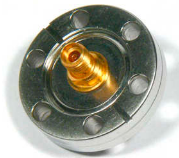
The Vacuum side of the 40 GHz Feedthrough, mounted on a 16CF flange. Please note that normal SMA connectors will fit, but might damage the Feedthrough. Only the nut must be turned for fixing the connector, never the connector itself.
