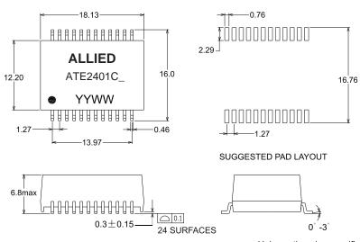
Unless otherwise specified all tolerances are:  $\pm 0.25 \text{ in mm}$
