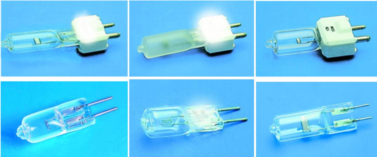
Above Amglo lamps represent various styles currently supplied to OEM's in operating room theater lighting. Lamp wattage ranges from 20-watts to 250-watts and voltage ranges from 12V to 120V. Filament types include C-8, CC-8, C-6, CC-6, C-2V, CC-2V, and C-Bar designs. Lamp glass is clear or frosted. A variety of lamp bases are utilized including SC Bay, DC Bay, Bi-Pin, and special Ceramic.
