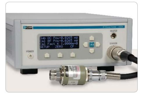
Thermistor RF power sensors are universally recognized as the most accurate means to measure and transfer RF power. The TEGAM Model 1830A was designed to operate with all types of thermistor RF power sensors while further reducing uncertainties. It combines a modern DC substitution bridge with a precision measurement system to provide consistent, calibrated RF power readings manually or automatically.
