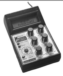
send the changes via the program button and the DigiDrive<sup>™</sup>II is set to more effectively control the motor for the intended application.
